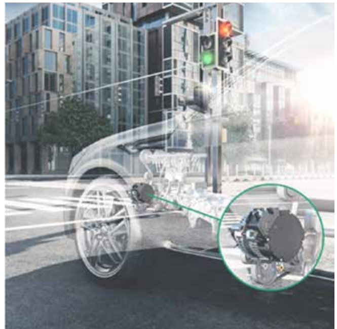
Fig. 1. Test case: SEG Automotive's Boost Recuperation Machine (BRM) system – one of the leading 48V machines on the market and already deployed in over one million vehicles on the road across the globe.
