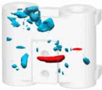
Fig. 5. Detail of predicted porosity defects due to shrinkage and air entrapment compared with X-ray analysis and destructive testing.
