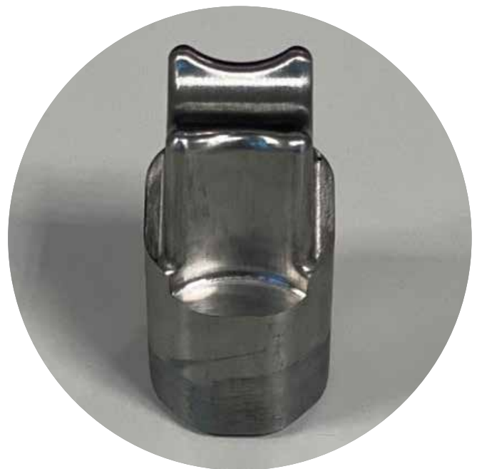
Fig. 13. Completed plug after machining.
